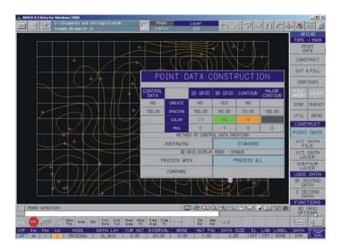
The topographer system is designed to create contour maps and 3D surface models from raw X,Y, Z data. Data may originate as surveying data, USGS data, or be generated by the user. Also, once a a existing and proposed model has been created of a particular site, it is possible to perform cut and fill calculations. Create quick, easy and accurate contour lines automatically You can create either "Mesh" or "Cake" 3D Terrain models from your contour data.
